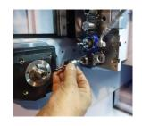
The traditional system for tool change in driven tool holders is not safe.
