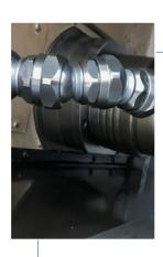
2. ARTICULATED STEEL FLEXIBLE DISTRIBUTION TUBES FOR MACHINING WITH LOW, MEDIUM AND HIGH-PRESSURE COOLANT
