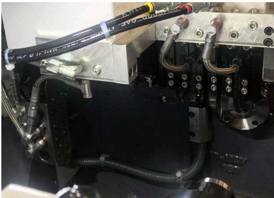
MICRO flexible tubes, banjos and quick connections fittings installed in a CITIZEN L12
