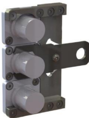
SP-BS-01-05 + SP-BS-03-04 blocking the middle non-cartridge type rotary tool holder in the main tool post STAR SR-20 / 32
