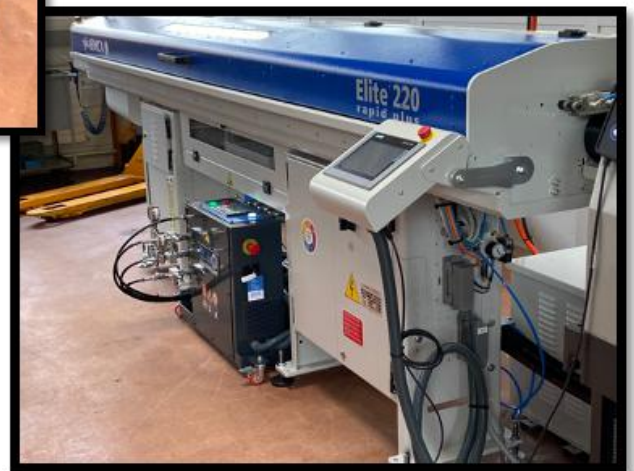
SCS-200 OIL 135Bar 24L/min.
